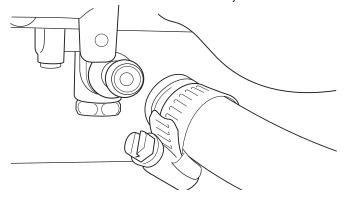
16. Remove existing jet from lower carburetor inlet.
